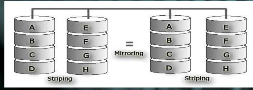
Striping – "segmenting logically sequential data, such as a file, and storing them on different disks"
